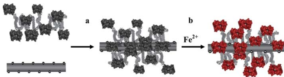
Fig. 1 The design of the protein-polycation-clay composites. (a) A complex of apo-mFd dimers (dark grey) and polycation (light grey) adsorbs on montmorillonite clay (rectangular sheet). (b) The composite (apo-mFd dimers and polycation complex on montmorillonite) chelates \text{Fe}^{2+} under reduced conditions (apo-mFd turns red upon chelation).
